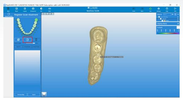
The software will register the Encode library and provide an automatic Encode suggestion. Please compare and verify the geometry of the Encode suggestion with the Encode scan in the middle. Select "OK" confirming that you have verified the Encode suggested and agree to proceed with registration and conversion.
