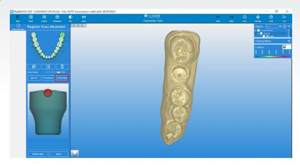
Start the registration process by selecting points on the Encode surface on your scan on the left window and matching corresponding points at the same location on the Encode cross-section window on the right. Once done, select "Fit."
