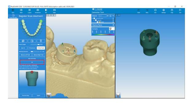
Ensure that the Encode is registered correctly and there is no rotation or alignment issues. Select "OK" if satisfied with the registration and alignment, or select "Edit" to change the "Fit By Points" registration.
